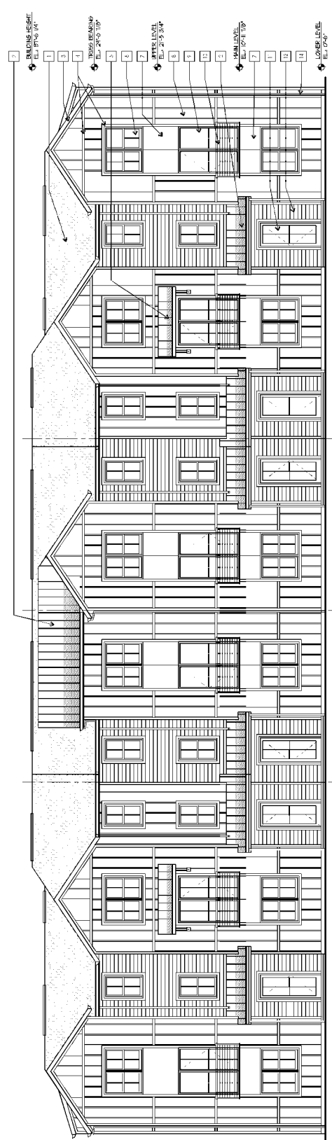
3-STORY FRONT ELEVATION - 6 UNIT BUILDING 3/16" = 1'-0"
