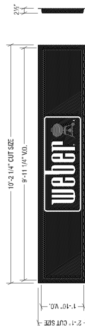
F TWO(2) PAN FORMED CLEAR POLYCARBONATE FACES W/ BLACK & RED VINYL GRAPHICS SCALE: 3/8" = 1"
