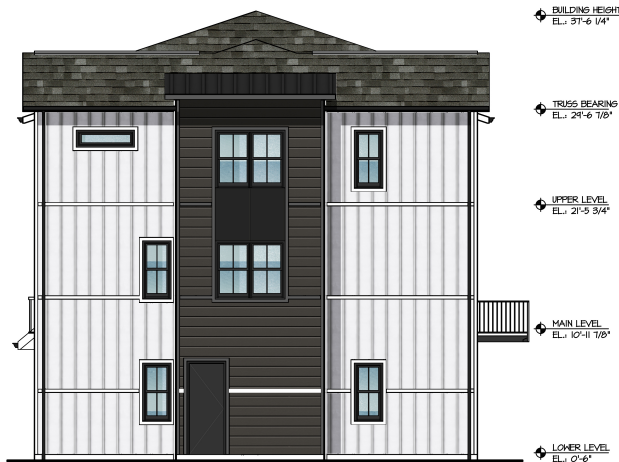
3-STORY SIDE ELEVATION - UNIT A 3/16" = 1'-0"
