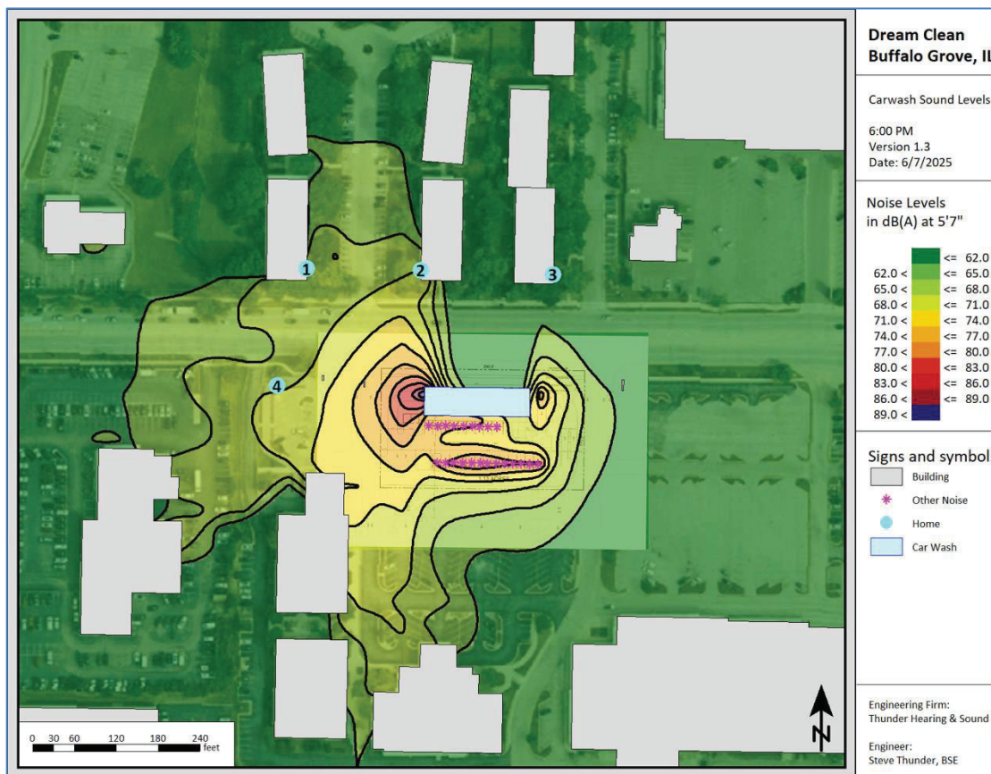
FIGURE 5 – Projected car wash sound level contours at 6:00 PM.
