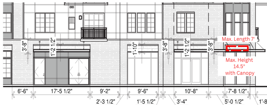
ENLARGED SOUTH EXTERIOR ELEVATION
